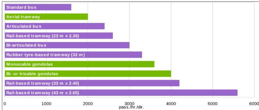
Figure 2: Capacity pphppd (passengers/hour) of typical urban transport systems (Bergerhoff and Perschon 2013)
