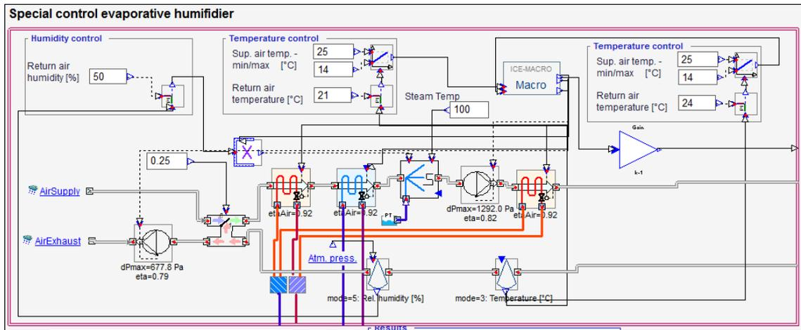
Fig. 6 - Modeling of the ventilation system
