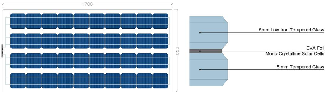
Figure 8. PV glass designed for the Parking Lot: plant and section. Source: Onyx Solar
