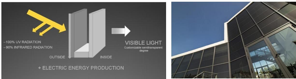
Figure 4. PV Curtain Wall scheme and real integration in Guadalhorce Headquarters, M3laga (Spain). Source: Onyx Solar
