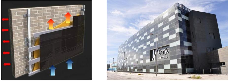
Figure 3. PV Ventilated façade scheme and double Skin PV real integration in Genyo Building, Granada (Spain). Source: Onyx Solar
