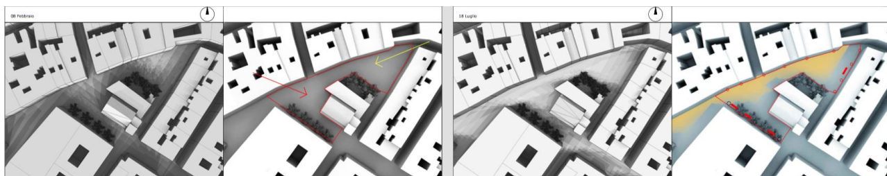
Figure 2 Sun shadow maps for 4 thresholds, with annotation of over lit and under lit zones and wind distribution, in Piazza della Pomposa, Modena.
